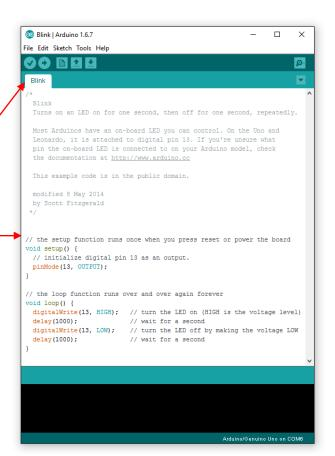
sketch is to blink a LED connected to the board at a rate of 1/2Hz (one second on then one second off).
